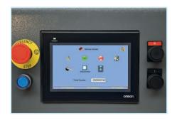
The **T.towel** has a PLC based control system. Operating the machine is done through an easy to use 7" color touchscreen. The control system needs a high computing power, therefore TEXFINITY has chosen OMRON. This powerful control leads to more precise folding, which has been clearly proven in comparative tests. Thanks to the responsive touchscreen of high resolution, making and changing folding programs becomes very easy.
