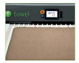
Pieces are put on the intake conveyor belt. This conveyor belt starts running once the piece is detected or after manual activation with a button at the side of the machine.
