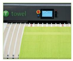
The **T.towel** is provided with a special feature to fold pieces that need extra corrections before being folded, like fitted sheets. After placing the sheet on the feeding table and pushing the button, the piece runs inside the machine and makes an automatic stop for correcting the tail end of the piece. Then, the operator pushes the button a second time so the folding process can start.
