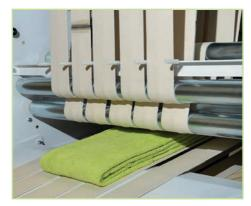
The **T.towel** is equipped with two cross fold sections. Each cross fold is made by reversing belts in combination with an air pulse. The result is a very precise and tight fold.
